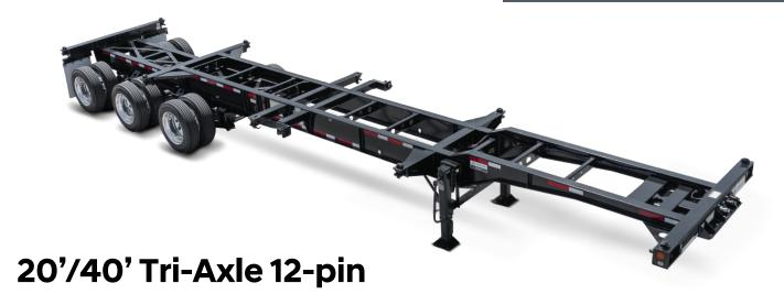
**Closed Length Extended Length** Overall Width Capacity 20' Capacity 40' GVWR 20' GVWR 40' Tare Weight 32' 1-1/4" 40' 6-3/16" 96" 66,400 lbs 74,400 lbs 77,000 lbs 85,000 lbs 10,600 lbs
